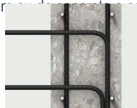
Traditional slab-to-wall construction joint
