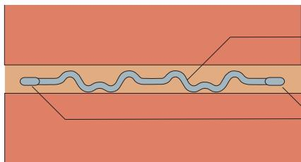
If applied to dry bricks or blocks, only the modified cross wires are in contact with the masonry; the longitudinal wires are elevated. When the next masonry unit is lowered, the mortar layer disperses around the steel, leaving the reinforcement fully surrounded.
