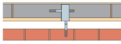
WP2 Windpost with SDN and SNS Ties in Cavity Wall
