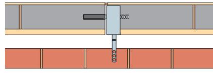
WP2 Windpost at Vertical Movement Joint in the Inner Leaf of Blockwork with Debonded Ties Across the Post
